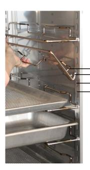
Some cabinet models are equipped with adjustable tray slides. Adjust tray slide positions by inserting "J" end of slide into upright key hole.
